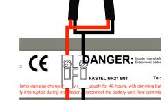
Next wire the spot lamps into the connector block for the emergency inverter. Ensure polarity is correct otherwise LEDs will not illuminate.
