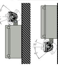
7. The lamps can easily be adjusted by hand and should be aimed to provide an even light distribution on the floor in accordance is BS5266. Once Adjusted the lamps must be locked in position.
