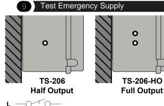
**9.** To test, briefly fail the supply to illuminate the spot lamps from the internal battery. The indicator LED will be extinguished to show that the mains has been disconnected.
